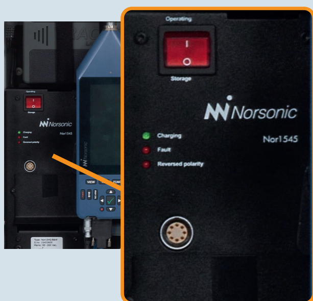
Figure 3: Status LEDs and Operating switch
